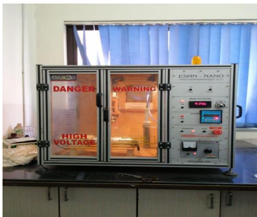
Figure 2: Actual setup of Electrospinning machine
