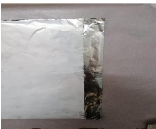
Figure 5: Image of obtained electrospun fiber on aluminum foil
